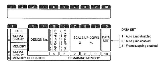
Example 1: Setting mirror image "P", with a scale factor of 100%, when using a TAJIMA tape
