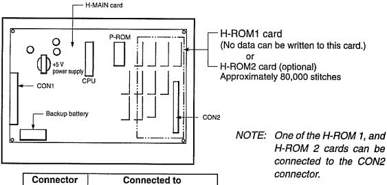
Connector Connected to
