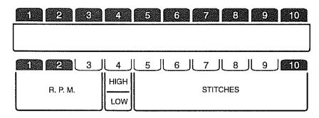
Example 1: Setting the high speed as 530 r.p.m. and the low speed as 400 r.p.m.
