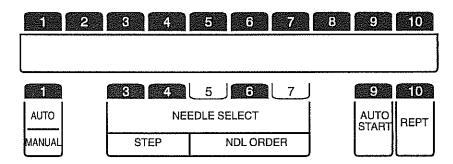
Example 1: Changing the needle bar selection setting from 1, 2 to 3, 12, 1
